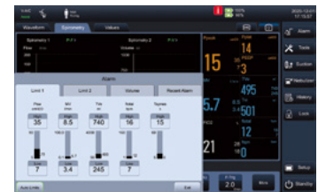
Automatic alarm limit
